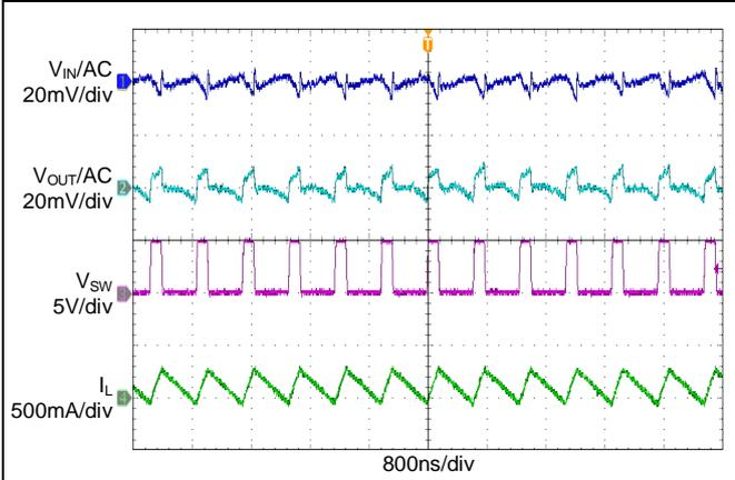
Figure 18. Steady State with Light Load
