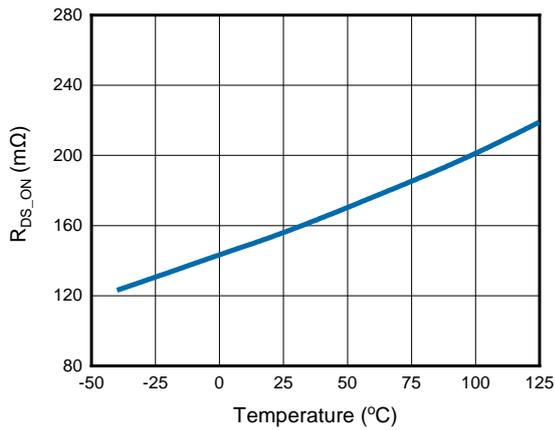
Figure 3. Low-side FET ON Resistance vs. Temperature
