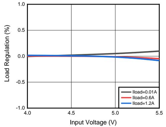
Figure 17. Line Regulation (V<sub>OUT</sub> = 3.3V)
