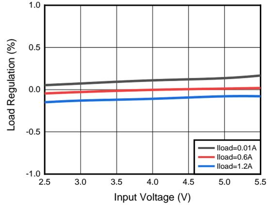
Figure 15. Line Regulation (V<sub>OUT</sub> = 1.2V)
