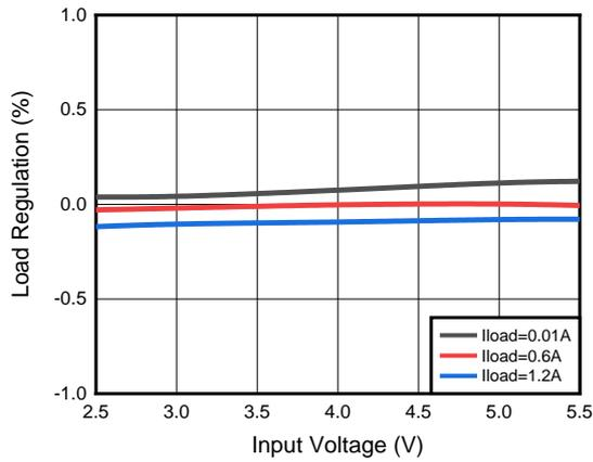
Figure 16. Line Regulation (V<sub>OUT</sub> = 1.8V)
