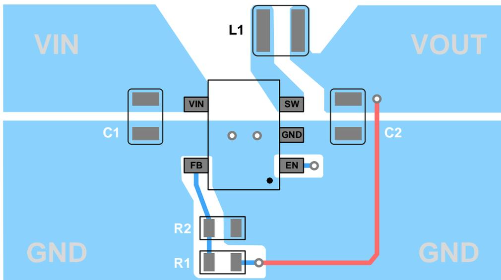
Figure 38. Typical GD30DC1109 Example Layout
