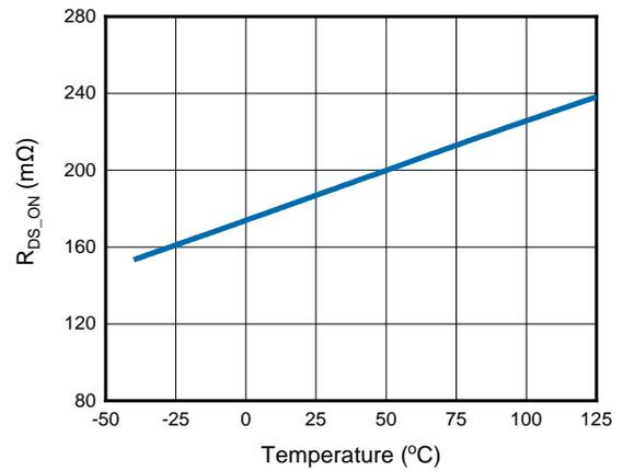
Figure 4. High-side FET ON Resistance vs. Temperature
