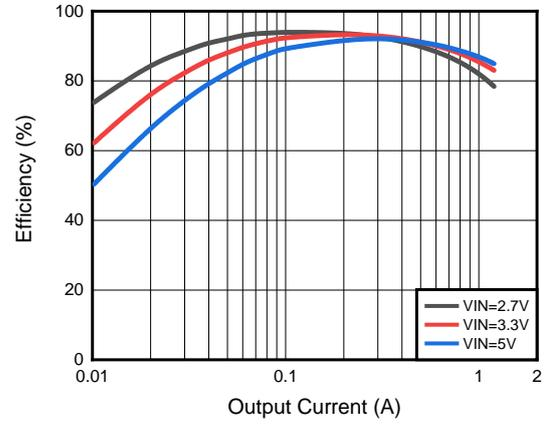
Figure 9. 1.8V Output Efficiency
