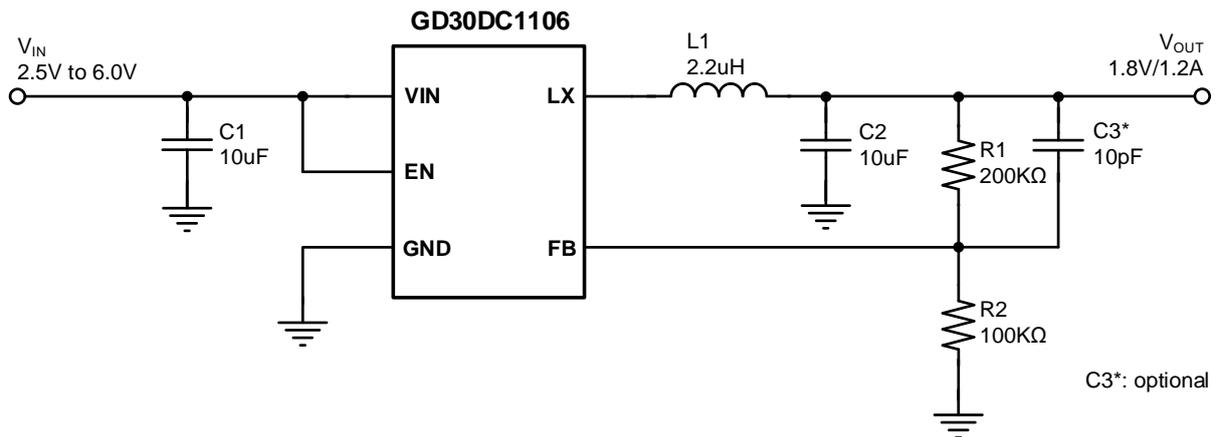
Figure 6. 1.8V, 1.2A Reference Design
