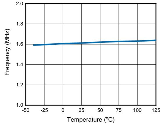
Figure 2. Switch Frequency vs. Temperature
