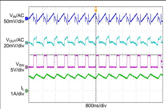
Figure 19. Steady State with Heavy Load
