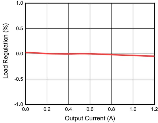
Figure 14. Load Regulation (V<sub>OUT</sub> = 3.3V)
