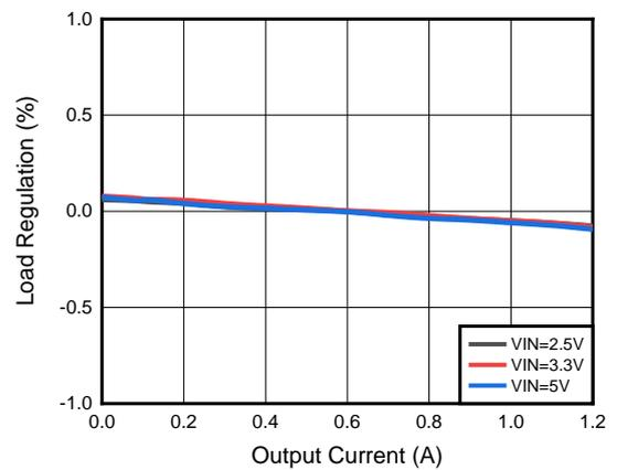
Figure 13. Load Regulation ( $V_{OUT} = 1.8\text{V}$ )
