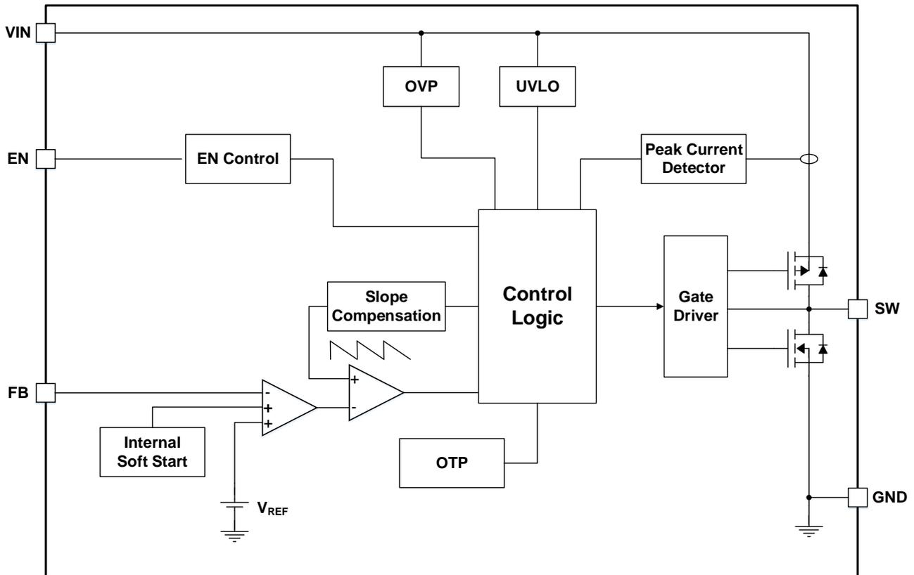
Figure 5. GD30DC1109 Functional Block Diagram
