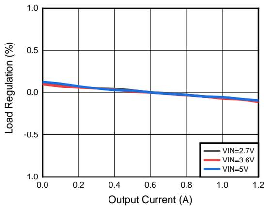
Figure 12. Load Regulation ( $V_{OUT} = 1.2\text{V}$ )
