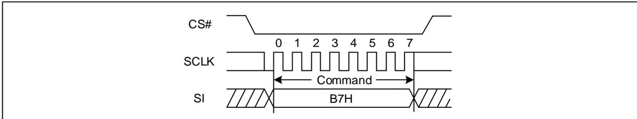
Figure 10 Enable 4-Byte Mode Sequence Diagram (QPI)
