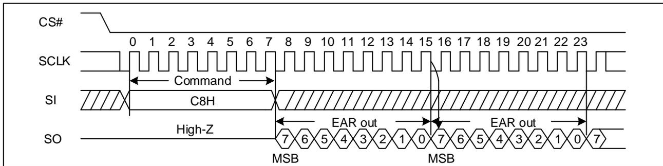
**Figure 34 Read Extended Address Register Sequence Diagram (QPI,  $f_{SCLK} \leq 104\text{MHz}$ )**
