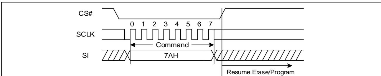
**Figure 75 Program/Erase Resume Sequence Diagram (QPI)**
