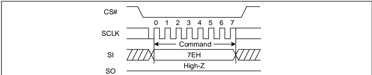
**Figure 89 Global Block/Sector Lock Sequence Diagram (QPI)**
