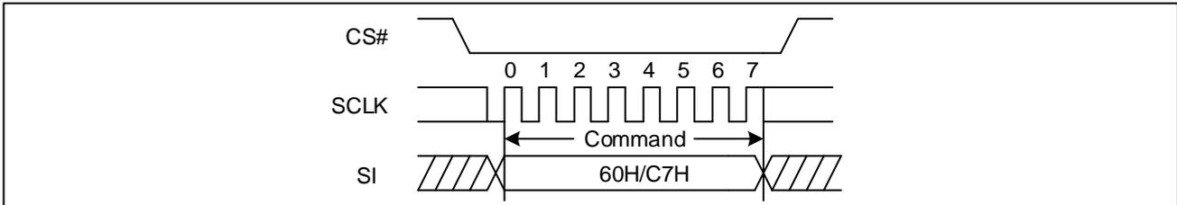
**Figure 60 Chip Erase Sequence Diagram (QPI)**
