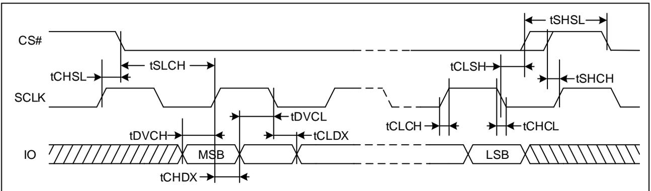
Figure 102. Serial Output Timing (DTR)
