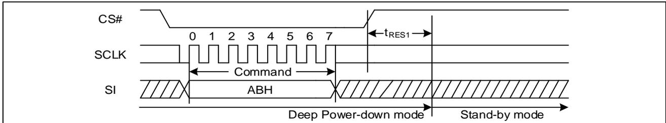
**Figure 66 Release Power-Down Sequence Diagram (QPI)**
